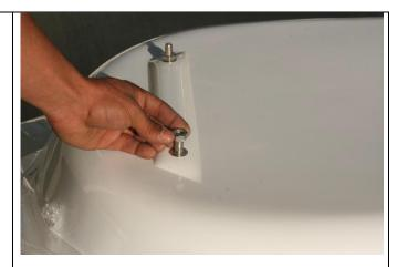
3. Loosely attach the bars to the base of the tub. Don't tighten fully as you will need to adjust later. If your tub is double ended, it will only have two straight bars, no V bars as shown in this generic photo.
